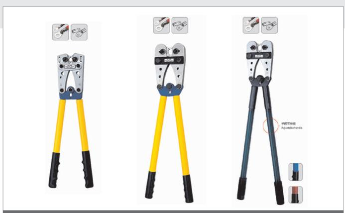
The crimping tools is used for non-welding and standard electrical connection. The mould of the crimping dies is made of SCM-40 hardest tool steel, It is with the characteristics of long life, accurate bore diameter and good crimping effect
